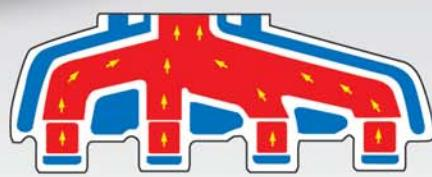
Our fully tuned design will reduce turbulence and enhance flow for added performance. An extra 30% water cooling area will help reduce temperature in the exhaust exit area allowing for longer gasket life.
